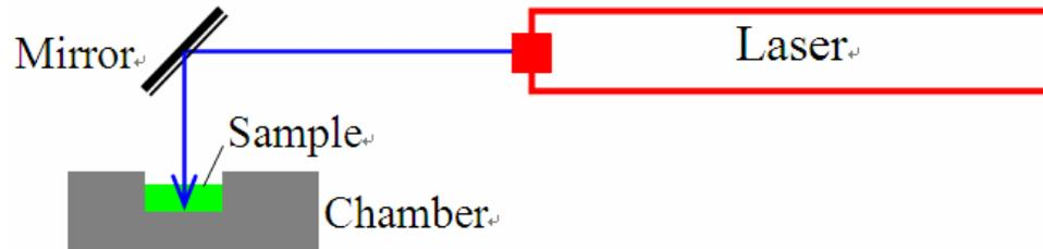
Most of our *in vitro* CALI was done in this simple system shown in the diagram irradiated with 800 mW for 45 mins. The irradiation source is a Spectra
